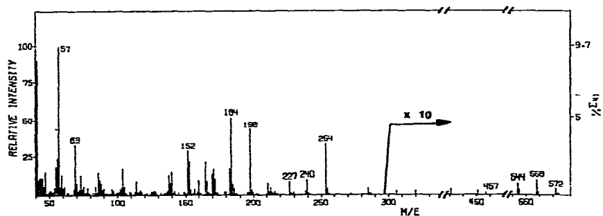
Fig. 4. Mass spectrum of TAB-cysteine-homocysteine mixed disulfide.
